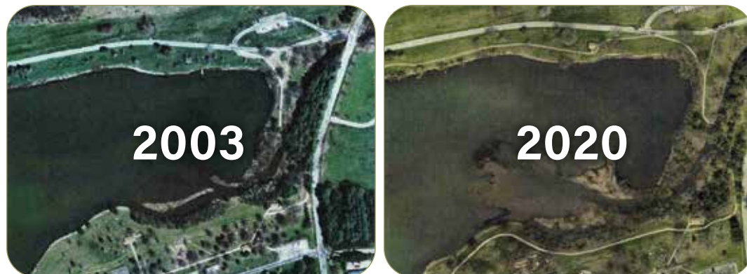
Figure 1. Drone images of Mammoth Lake in 2003 and 2020. Note the formation of the large sediment peninsula in the 2020 photos. Photos taken from the Westmoreland County tax map system.
